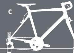
Adjust position of rear hub according to your wheel base. Place rear drop-outs on rear hub with correct rear axle adapter. Tighten your rear axle.
