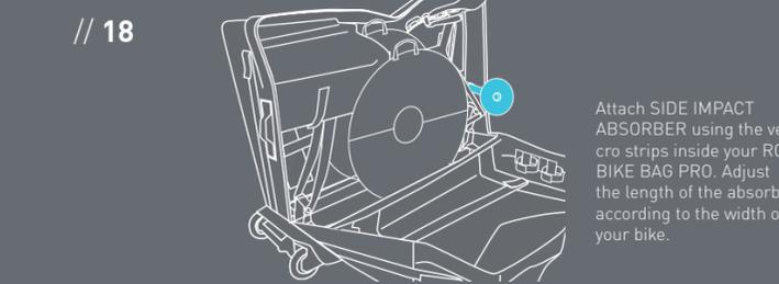
Attach SIDE IMPACT ABSORBER using the velcro strips inside your ROAD BIKE BAG PRO. Adjust the length of the absorber according to the width of your bike.
