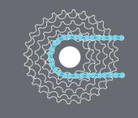
Chain on smallest sprocket
