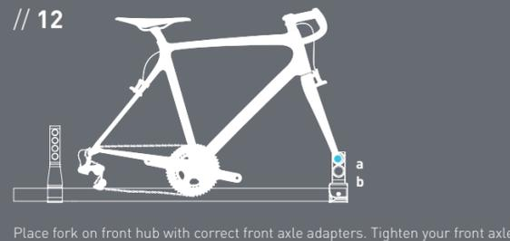
Place fork on front hub with correct front axle adapters. Tighten your front axle.
