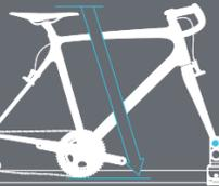
Maximum length from seat top to bottom of chainring is 86cm. Maximum wheel base is 106cm.
