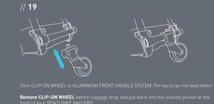
Click CLIP-ON WHEEL to ALUMINIUM FRONT HANDLE SYSTEM. Pin has to go into feed holes!
